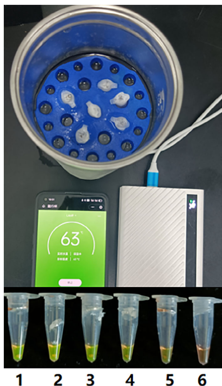
Figure 4. Field apparatus and loop-mediated isothermal amplification (LAMP) results. The reaction tubes are placed in heated water in a commercial insulated cup, whose temperature is controlled by a phone application. Insect tissues are placed directly into the reaction tubes. Tubes shown at the bottom are: Phthorimaea absoluta larvae (1, 2), P. absoluta adults (3–5), and sterile double-distilled water (ddH 2 O) (6).
